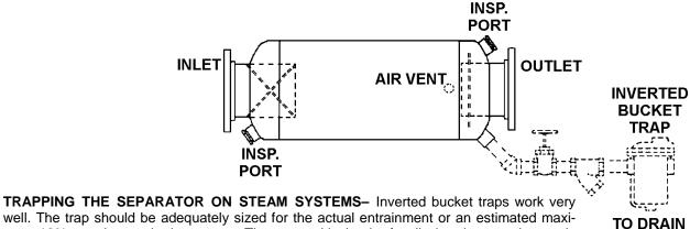
well. The trap should be adequately sized for the actual entrainment or an estimated maximum 12% entrainment in the system. The most critical point for discharging entrainment is during start up. To compensate for proper drainage a safety factor of 2-3 times should be used. Penn Brochure page C-7, D-7 shows a trap selector chart for most applications. The pressure rating on the rap should be checked to comply wit the separator requirements. The trap should be located below the separator drain.
