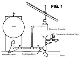
At the left shows the simplest and most practical installation since it provides ready drainage for most heating or process boilers. A dead boiler drain is also included. The boiler, piping, and blowdown valves would be provided by others.
