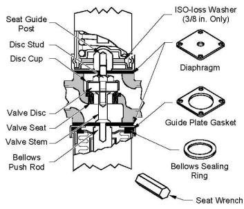
Figure 3: Diagram of 3/8" through 1-1/2" Valve
