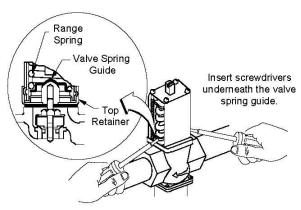
Figure 1: Manual Flushing
