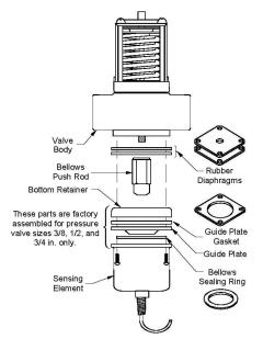
Figure 5: Guide Plate Gasket and Bellows Sealing Ring Identifications
