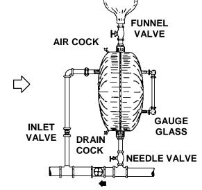
AS DIP FEEDER TO OPEN VESSELS Close inlet valve, open funnel valve and place over vessel to drip freely.
