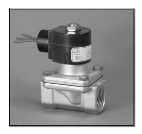
The S21 Series 2-way general purpose solenoid valves are of piloted diaphragm construction and are available in normally closed and normally open operating modes. They are available in a variety of pipe connections from NPT 3/8" to 2" There is an extensive range of options. This series is widely used in various industrial applications. For special applications, contact your Penn Separator representative. Penn Separator uses the following as standard.
