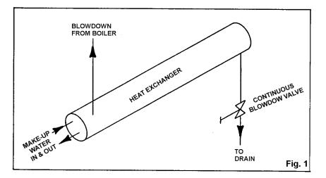
Using a U-tube heat exchanger with 50% make-up, at 60°F the drain water from the heat exchanger (cooled continuous blowdown) can be reduced to 110° F. The amount of heat recovered with this type system then becomes:
