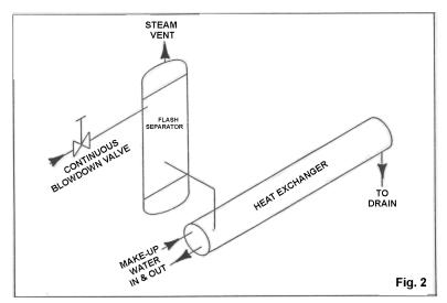
The amount of heat recovered in the 1st Stage is a function of the drop in pressure on the blowdown water. For our consideration let's use the 150 PSIG boiler going to a 5 PSIG deaerator. At these pressures a percentage of the blowdown flashes to steam. This percent is determined by the following formula:
