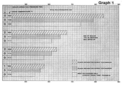
The head recovery in the 2nd stage then becomes enthalpy of water  $226.6^{\circ}F$  at 5 psig (195.33) - enthalpy at 100° (67.97) = 127.36 BTU's/# recovered with the heat exchanger. Therefore, 1761.43#/Hr. X 127.36 BTU's/# = 224,335.72 BTU's/Hr. recovered in the 2nd Stage. To get the total BTU's recovered add the 1st Stage and the 2nd Stage together. This gives a total of 581,041.41 BTU's/Hr. recovered from the continuous blowdown.
