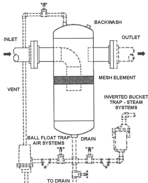
A Backwash connection is provided on all Mist Separators because mesh fouling can occur. By simply flushing the pad with water should provide sufficient cleaning. An increase in pressure drop through the unit is an indication that the element has become fouled. As an option body flanges or a manway can be provided for pad access, replacement, and removal.
