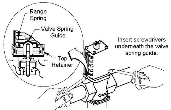
Figure 1: Manual Flushing
