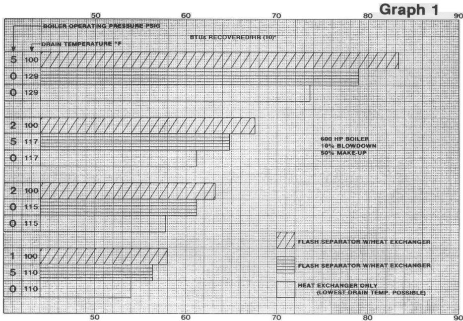
The head recovery in the 2nd stage then becomes enthalpy of water 226.6°F at 5 psig (195.33) - enthalpy at 100° (67.97) = 127.36 BTU's/# recovered with the heat exchanger. Therefore, 1761.43#/Hr. X 127.36 BTU's/# = 224,335.72 BTU's/Hr. recovered in the 2nd Stage. To get the total BTU's recovered add the 1st Stage and the 2nd Stage together. This gives a total of 581,041.41 BTU's/Hr. recovered from the continuous blowdown.
