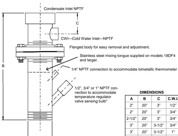
\* Temperature regulator valve sensing bulb to be installed in lower section so that mixed water temperature is sensed by bulb. Valve modulates to add sufficient cold water to lower drain water temperature. See Penn Brochure pages B-7 thru B-8.5 for further details.
